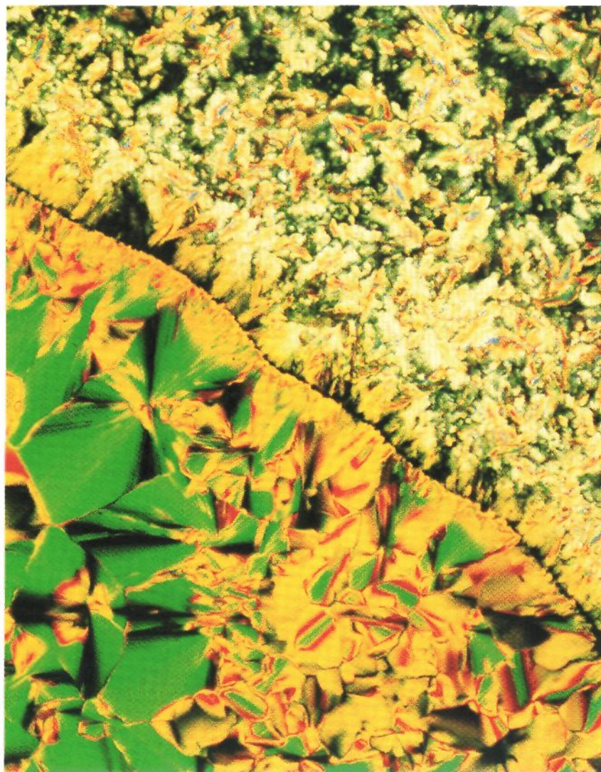
Figure 2. Photograph of a contact preparation showing the lack of miscibility of the O_h phase of 3 , N = 12 (bottom) with a D_{hd} phase of a square-planar copper diketonate complex (top) viewed with a polarizing microscope at 90 °C (polarizers oriented vertical and horizontal).
